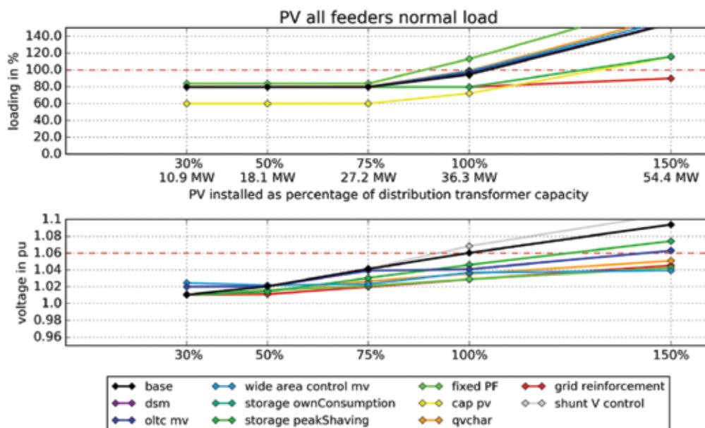
**Figure 8: Simulation results for the rural feeder in Bhopal with rooftop photovoltaic plants equally distributed along the feeder with normal load considered**
